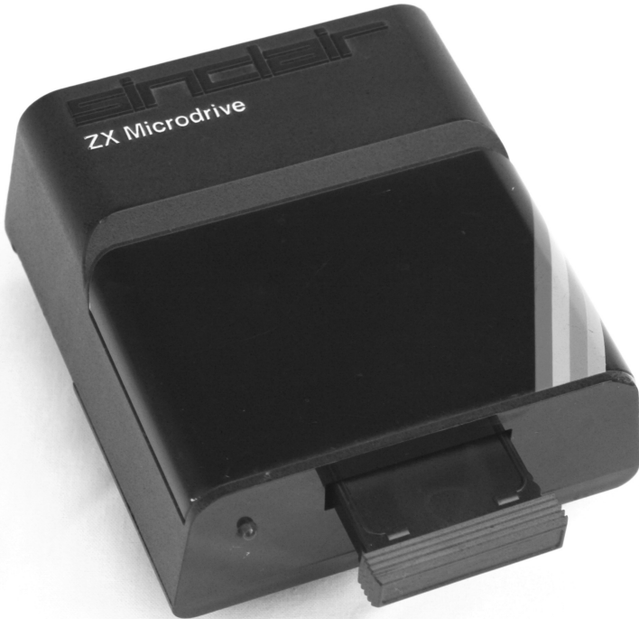
Fig 1.10 Microdrive cartridges contained a 15m spool of tape that whizzed around at two metres per second.
